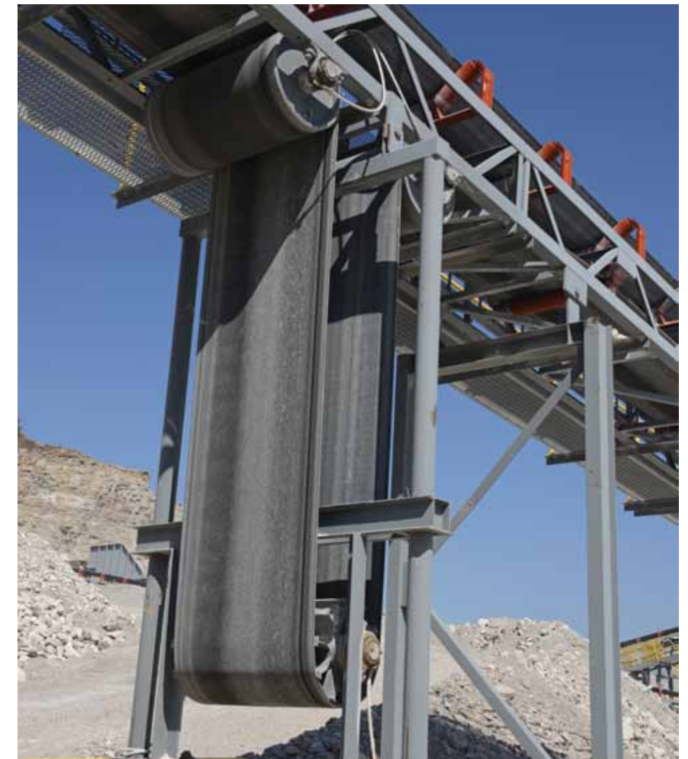
Baldor's Dodge Mine Duty Extra Drum and wing pulleys feature the proven High Endurance (HE) integral one-piece end disc design that can handle loads up to four times higher than standard CEMA drum pulleys.
