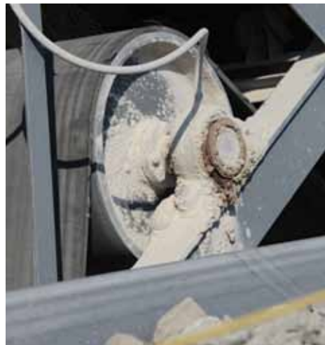
Baldor's Dodge Imperial-E spherical roller bearings feature a patented locking system that provides a concentric grip to the shaft for superior holding, with Type E mounting dimensions. Proven Trident seals provide maximum sealing protection and are extremely effective for harsh and dirty environments.
